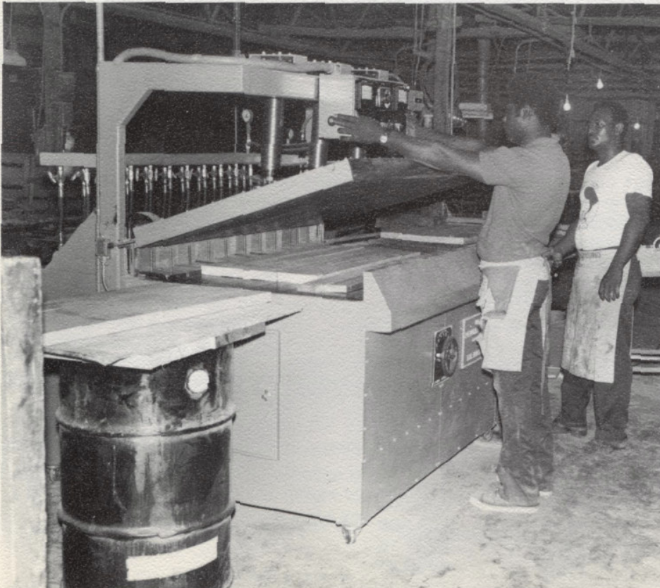
Figure 14: L&L radio frequency gluer. (Photo courtesy of L&L Machinery, North Wilkesboro, N.C.)
